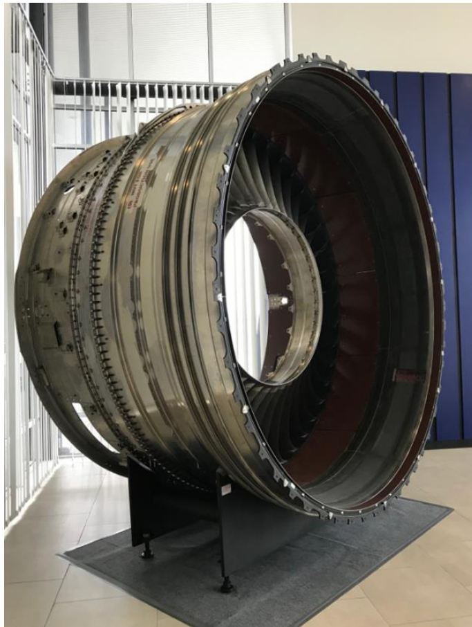
Figure 4: Rolls-Royce Trent 1000 engine fan case
